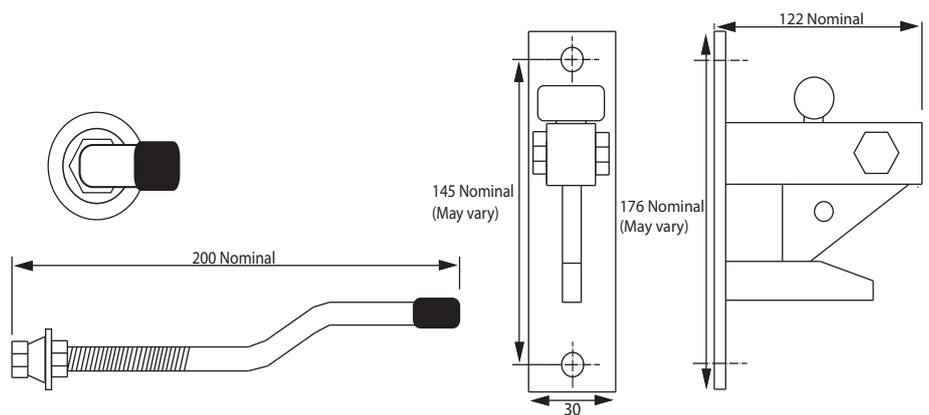
Gate latch and striking pin (Note, please state diameter of tube it is being fixed to). 3 x Lockinex A36 clamps are required to fix to the supporting tube. Relevant fixings/screws are also required separately to connect latch to A36's.
