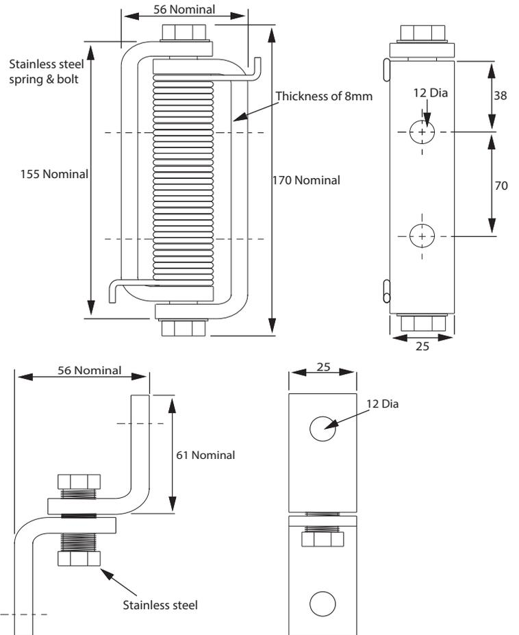
Gate spring set. Available with all mild steel components in galvanised or self colour (For welding). The suggested maximum weight of the gate 10kg. Use multiple springs if gate is heavier. Spring functions through 90 degrees max.
