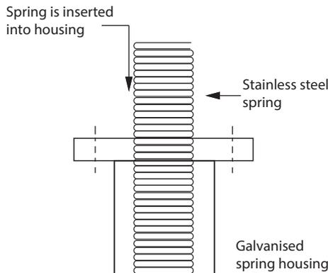
Slotted bolt locates onto leg of spring
